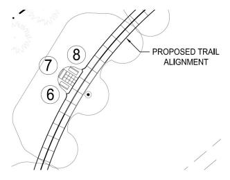
The proposed trail is 8 feet wide. The figure on the left shows the location of bench # 6-8 The half-round symbol with a black dot across from the benches shows the location of one of the future Solar light. Poles. All benches are to be located in the lighted area.
